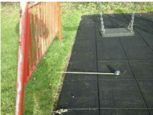
The surfacing width under each seat is less than 1.75 metres and fails the requirements of BS EN 1176 Part 2 Finding:
