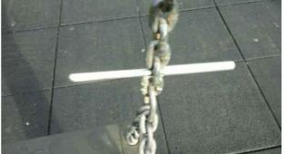
Finding: The chain openings are in excess of the 8.6mm as recommended by BS EN 1176
