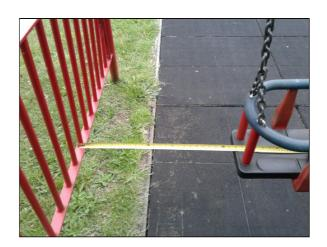
The surfacing width under each seat is less than 1.75 metres and fails the Finding:
